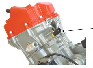
Install the water temperature sensor.
