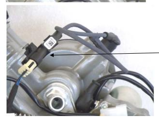
Connect the crank trigger sensor.
