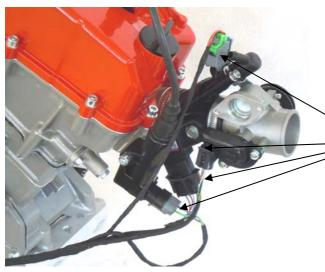
Connect the injector nozzle, throttle position sensor, MAP sensor and the ignition coil.
