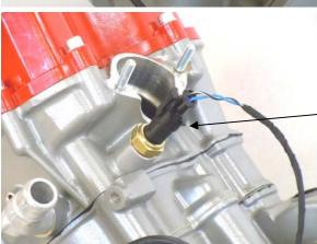
Connect the water temperature sensor.
