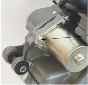
Connect the engine ground cable to the engine
