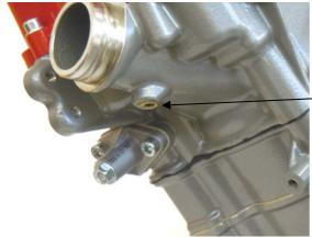
Close the hole with the screw plug Use Loctite 577
