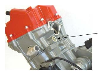
Remove the screw plug in the cylinder head.
