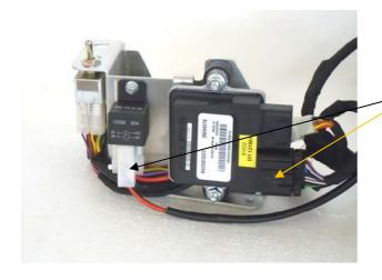
Install the reprogrammed or exchanged EFI ECU.
