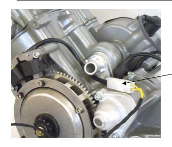
Connect the generator stator to the wire harness.
