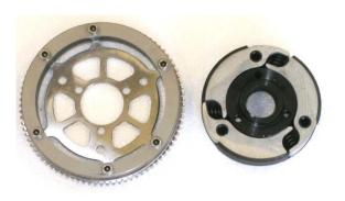
Now you can remove the clutch from the starter sprocket and change the complete clutch or just the clutch jaws.
