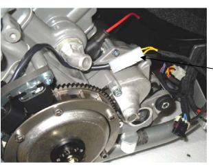
Connect the engine wiring harness with the generator.
