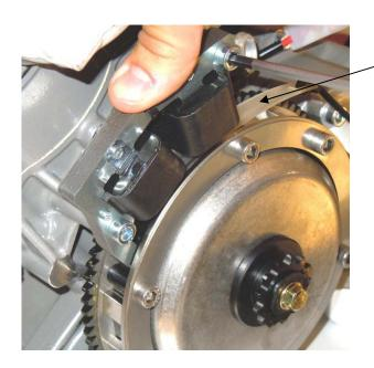
Slide the bent feeler gauge of 1.2mm between generator stator and the magneto.
