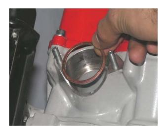
Put the primary tube gasket into the primary tube port.
