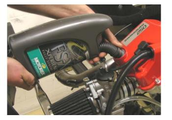
Fill in 0.4I 0W30 motor oil from "Motorex" into the engine.
