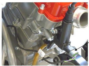
Connect the engine wiring harness with the ignition coil.
