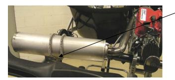
Install the exhaust silencer on a commercially available exhaust bracket (not included in the scope of supply).
