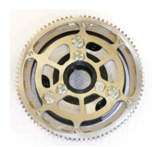
Mount the new clutch on the starter sprocket.
